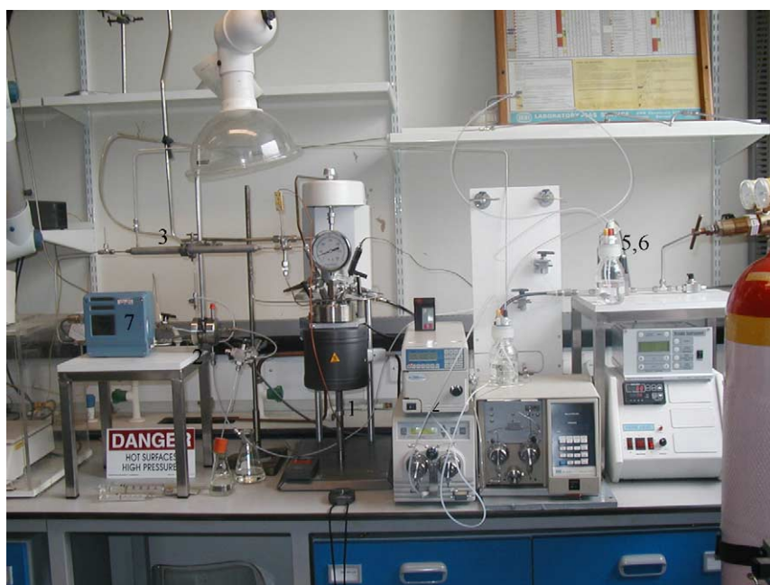
Fig. 2. Photograph of the continuous flow fluoruous biphasic experimental set-up.
